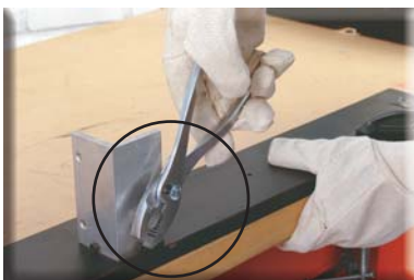
Pliers should not be used with nuts or bolts; a wrench will do the job better and won't deform the fastener.
