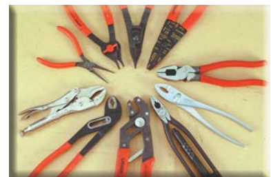
Use the right pliers for what you are doing (stripping, cutting, threading, setting terminals, etc.).
