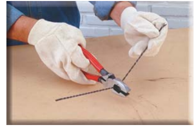
Do not fold the wire against the blade edges.
