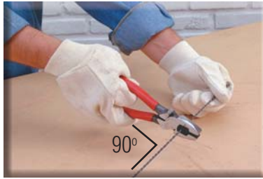
Always cut at right angles and never swing the pliers or snips from side to side.
