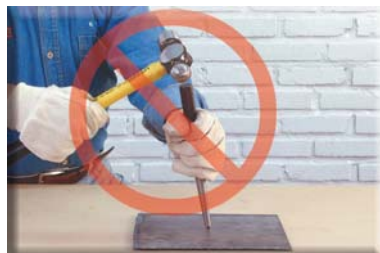
Never strike with the side of a hammer.
