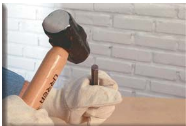
The head of a hammer for striking a chisel should be approximately 75% larger than the chisel.
