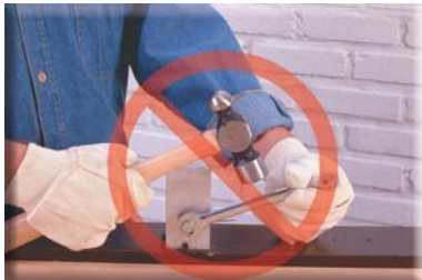
Never use a hammer on a wrench unless it is designed for such use.
