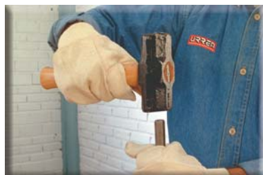
Always strike the heads of punches, chisels and nail sets squarely. Always strike so that the face of the hammer is perpendicular to the striking surface. Avoid grazing blows.
