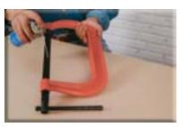
Always make sure that the center screw is clean and well lubricated.
