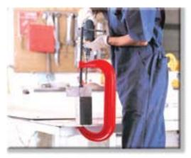
Swivel-tip screw adapts to the surface of the part to be held.
