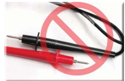
If any damage is detected on a test tip wire, replace it immediately.
