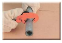
When using a pipe cutter, always mount it perpendicular to the pipe.
