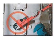
Do not use pipe or chain wrenches on square or hexagonal shapes; doing so can cause accidents, damage the part, or damage the wrench.
