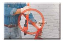
Never use a pipe wrench to bend, hoist, or lift a pipe.
