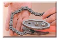
The chains on universal wrenches should be checked periodically for damaged pins or links.
