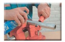
The pipe and pipe cutter should be lubricated to reduce friction.
