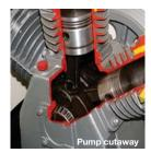
The 100% cast-iron TRI-MAX™ Series pump features simple splash lubrication for total reliability and a "W-3" finned cylinder configuration that provides 360° cooling. Lower RPM's and large-diameter finned copper tubing between stages, means they will run cooler, which ultimately achieves maximum compressor efficiency with less moisture contamination.
