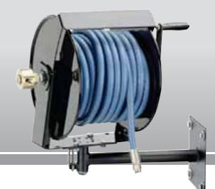
**COXREELS®** SM Series "Swivel Mount" hand crank hose reels swivel on demand in the direction your work takes you and locks in eight different positions as desired. Like the 100 Series, the SM Series is lightweight, compact and versatile with a working pressure up to 4,000 PSI. The "U" shaped base and hose control bar together add strength and rigidity while keeping the hose from slipping off the side discs. Add the SMK-202 wall mount bracket for swiveling mounted positions.
