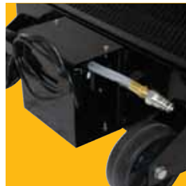
Electric Pump Evacuation System When full the reservoir is emptied using the 10' quick connect evacuation hose and the 110 V cap electric pump evacuation system mounted in the rear of the drain. The pump transfers fluid at a rate of 5 gpm. (Note: The transfer rate can vary based on fluid temperature.)
