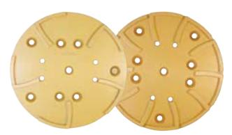
Designed for grinding concrete. They are excellent for aggressive stock removal and give rough concrete surfaces the smoothest finish in the quickest time. Can be used on single-head floor machines and may also be attached to Pearl's 11" Hexplate™ for use on the GRM11.
