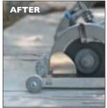
VACUUM REQUIREMENTS: SawVac™ will work with any vacuum, but for optimum efficiency use a vacuum rated at or above 11.5 amps (1.75 continuous hp) or 110 cfm.
