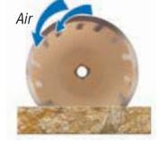
While the blade is cutting, the debris (swarf) is removed from the cutting path via the waved-core thus extending the life of the blade.
