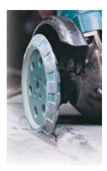
FOR CLEANING, ROUTING AND REPAIRING OF CRACKS IN CONCRETE AND MOST OTHER BUILDING MATERIALS.
