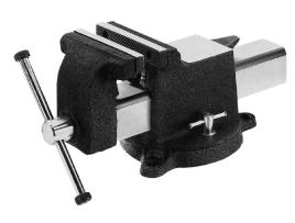
All Steel Utility Shop Vises are economically priced for various less demanding applcations. The entire vise body is constructed using structural cast steel. The bar covers the continuous rolled main screw. Each vise is equiped with replaceable hardned steel serrated jaws and built-in pipe jaws. The 360 degree swivel base features two (2) lock downs.
