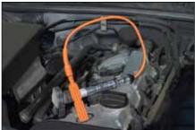
Test coil directly to ground
