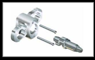
causing the ramp to lift the steel ball, lifting the hammer assembly until the dog teeth no longer engage the anvil, and the hammer is free to spin again. The hammer then springs forward to the bottom of the ball ramp, and is accelerated by the input shaft, until the dog teeth contact the anvil again, delivering the impact.
