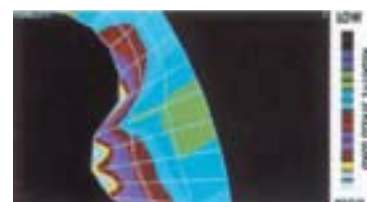
First Generation. While stress is relieved on the fastener corner, there is no significant improvement in relieving concentrated stress on the inside surfaces of the socket.
