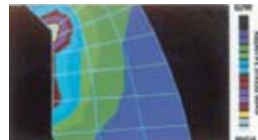
Conventional. This Finite Element Analysis display shows that ordinary sockets create extremely high stress loads at the fastener corner and at the socket's inside corners. The illustration shows that this stress is concentrated in a very small area.
