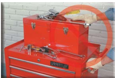
Never move a cabinet if it has parts or tools on top of it.
