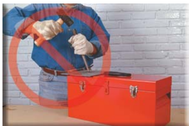
Never use tool boxes as supports for striking or drilling objects.
