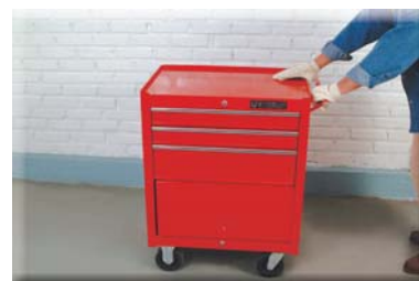
Never pull a mobile cabinet, always push to move it, and make sure that the floor underneath you is not slippery or wet from a spill.
