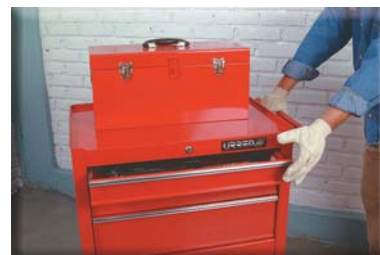
Make sure that all sliding shelves and drawers in the cabinet are closed before moving it.
