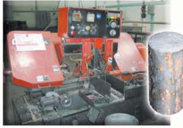
2A. Cutting the steel
