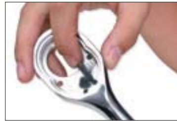
5. Position the spring for that catch hook (with the larger diameter against the hook).
