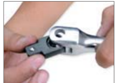
3. Insert the drive and washer into the handle fork.
