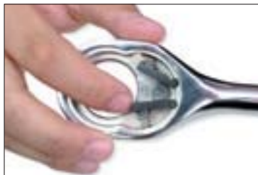
7. Position the second spring in the same manner as the first one.
