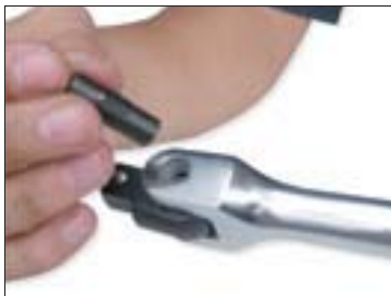
4. Insert the bolt into the handle borehole.
