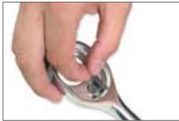
4. Place one of the catch hooks in its borehole (the hook's groove should be against the ratchet handle body).
