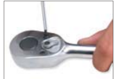
9. Insert the screws and tighten securely.
