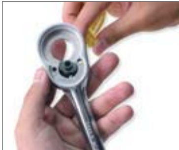
4. Maintain pressure on the bearing while you insert the cam into its place (drive facing down and teeth toward the borehole for the gear).
