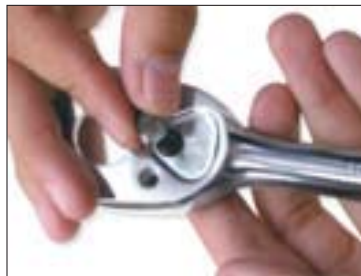
5. Insert the lever into the cam in the back of the ratchet.
