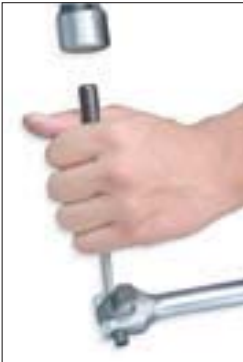
1. Remove the damaged kit, using a hammer and punch.
