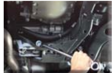
When changing the oil filter in a vehicle, first drain the engine oil; do this when the engine is not too hot.
