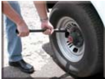
Loosen the wheel nuts about 1/4 turn with a wheel wrench before jacking up the vehicle.
