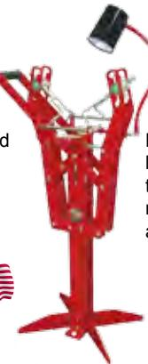
Passenger and light truck tire spreader minus gas spring and rollers
