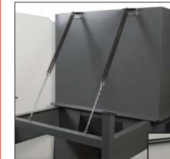
Flip Top (left) cabinets feature springs to assist the operator in opening the lid of the blasting unit.
